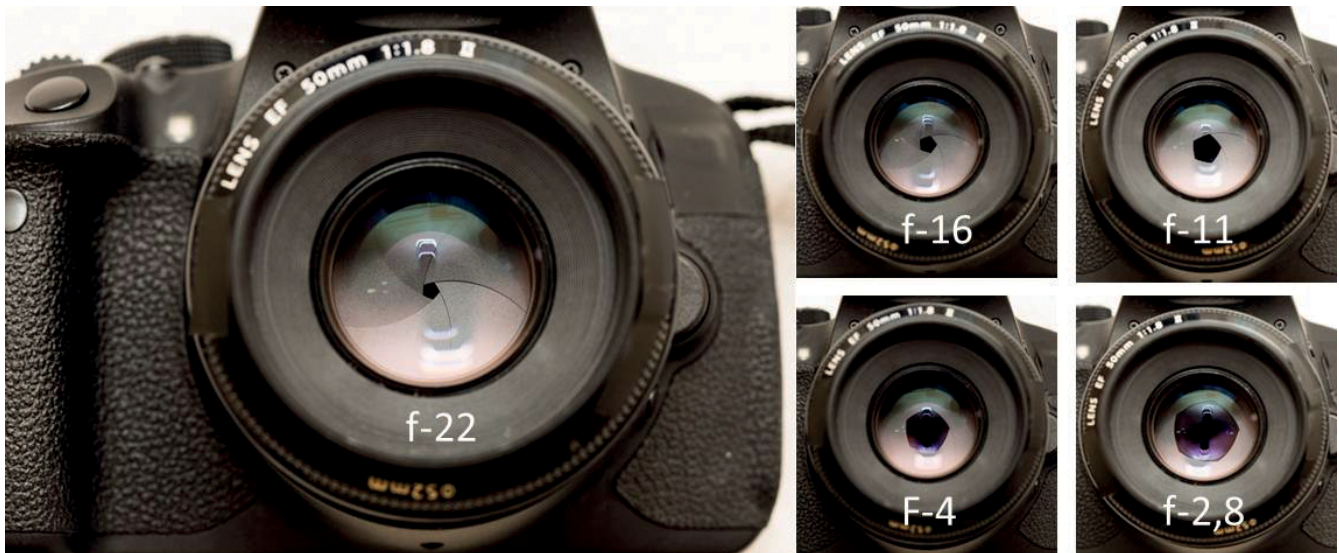
Figure 2. Aperture sizes. Small aperture ( f -22), less light strikes the image sensor. Large aperture ( f -2.8), more light strikes the image sensor.
